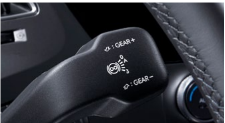
Auxiliary Brake and Manual Gear Shifter
