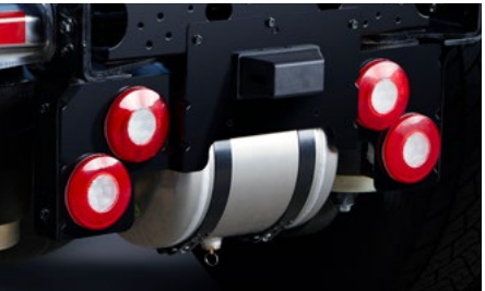
LED Rear Combination Tail Lamps The tail lamps feature LEDs for enhanced visibility.
