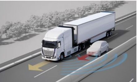
Blind-Spot Collision Warning (BCW) BCW is a driving safety function that warns drivers not to collide with rear-side vehicles.
