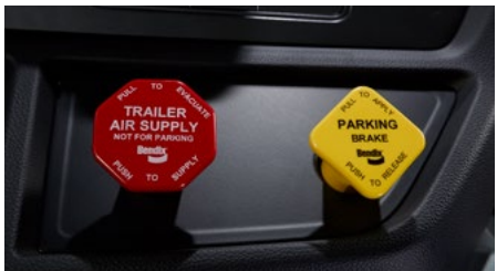
Trailer Air Supply and Parking Brake Switches
