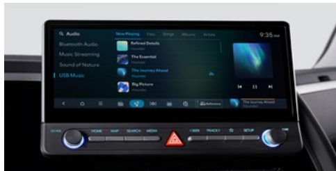
Intuitive 12.3-inch Touchscreen Directly below the head unit, a row of physical buttons flanked by rotary control dials serves as one-touch shortcuts to access the most commonly utilized functions.
