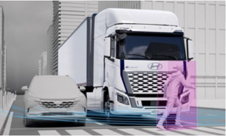
Forward Collision Warning-Near (FCW-Near) FCW-Near provides a warning on detecting the risk of forward collision with nearby objects in the blind-spot while driving at low speeds.
