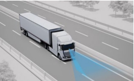
Lane Departure Warning (LDW) LDW alerts driver when the vehicle drifts out of its lane without signaling.
