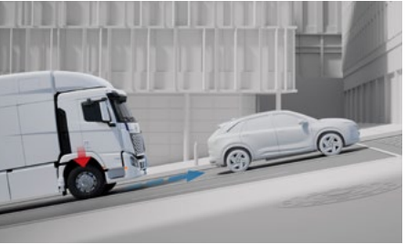
Easy Hill Start System (EHS) When stopped on an incline, EHS prevents inadvertent rollback by releasing the brakes only after applying pressure to the throttle pedal.
