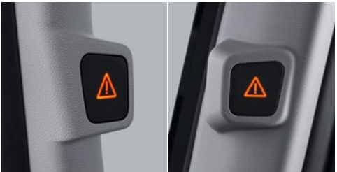
BCW* & BCW-Near Indicators The BCW & BCW-Near indicators are positioned on both front pillars for optimal visibility. * Blind-spot Collision Warning
