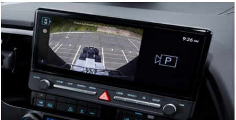
Deck View Monitor Equipped with an extra-wide-angle lens, the screen provides a real-time rear view video feed.
