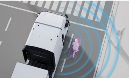
Blind-Spot Collision Warning-Near (BCW-Near) BCW-Near is a driving safety function that provides a warning if there is a risk of a collision with an obstacle approaching from the right blind spot (LHD reference).
