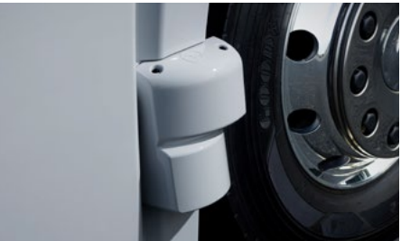
Side Radar Sensors Side-front radar and side-rear radar are encased in a sturdy protective cover, giving the driver an extra set of eyes in blind spots.
