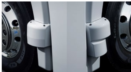
Rear Corner Radar Sensors (Passenger / Driver Side)
