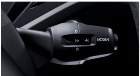
Gear Change Knob and Mode Switch
