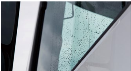
Water-repellant Door Glass
