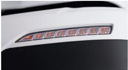
LED Clearance Lamps
